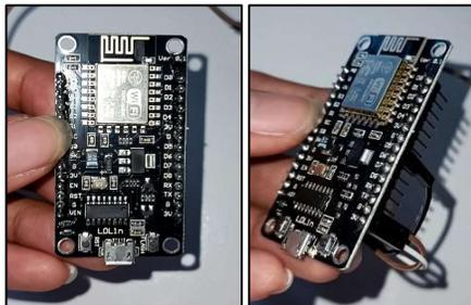
Gambar 9. Memasang Kabel Jumper Female to Female Ke NodeMCU ESP8266
