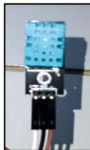
Gambar 12. Memasang Kabel Jumper Female to Female Ke DHT11
