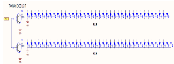
Gambar 31. Wiring Taxiway Edge Light
