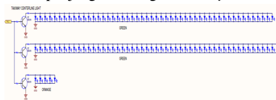
Gambar 32. Wiring Taxiway Centerline Light
